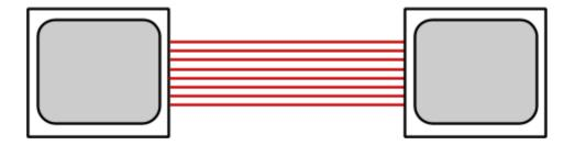
The more wires that a parallel communication medium uses, the more data can be transferred simultaneously.
